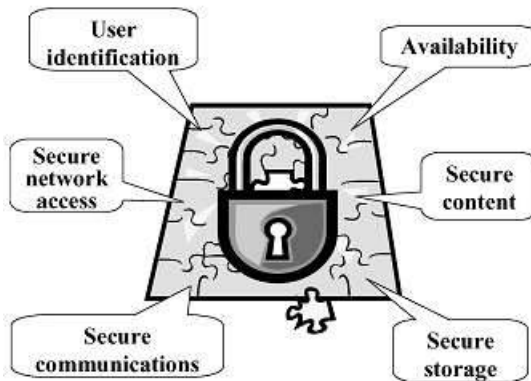
Fig. 3. Common security requirements of embedded systems.
